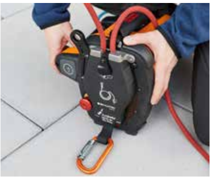
Semi-static working rope (SUPER STATIC 11.0) is placed in the ACX POWER ASCENDER
