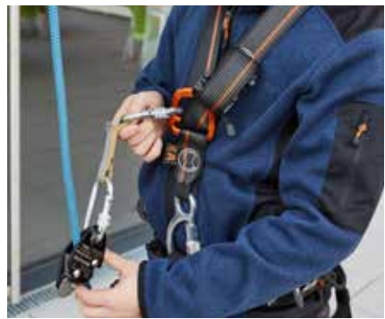
Backup rope is connected to the guided type fall arrester as per EN 353-2 and to the front attachment point of the harness
